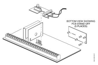
Connect field wiring to the desired trigger terminal on the trigger module (TRIG 1 = output 17; TRIG 2 = output 18) and the VTRIG +12V terminal.
